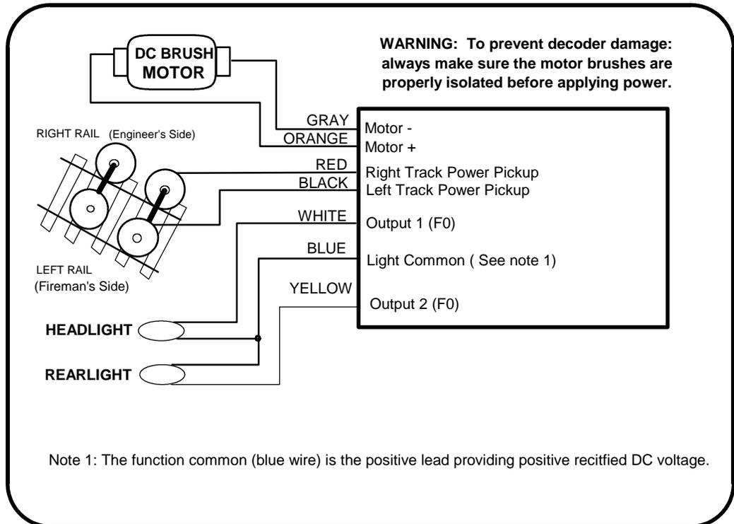
Before test running your newly converted locomotive on full power double check your wiring to make sure there are no pinched or broken wires. We see many decoders returned due to wires getting pinched between the body shell and frame causing shorts.
